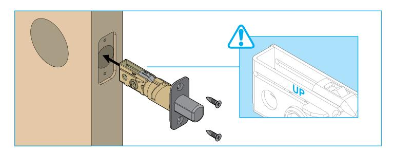
Locate latch with rectangular faceplate and insert screwdriver into latch cam.
