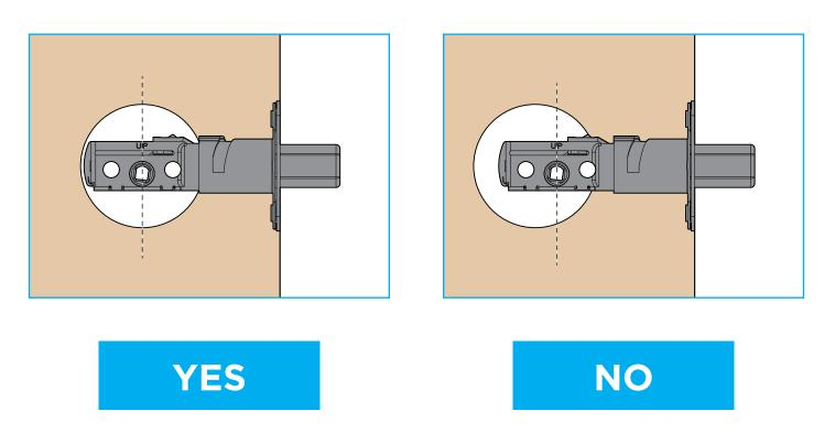
Install latch with the provided screws, making sure the word "UP" faces upward.
