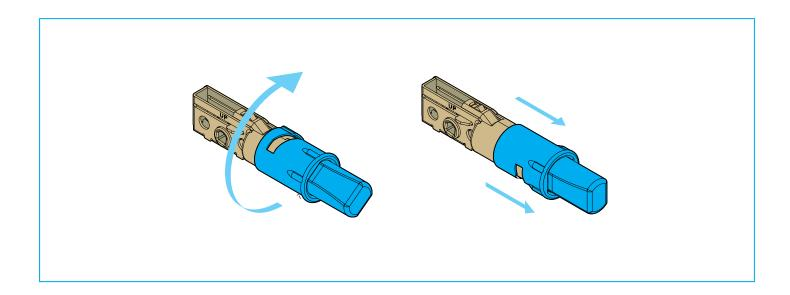
Use screwdriver to retract latch bolt.
